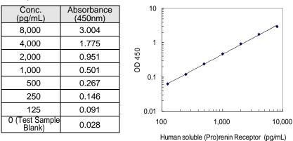
The typical standard curve is shown above. This curve can not be used to derive test results. Please run a standard curve for each assay.
