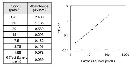
\* The typical standard curve is shown above. This curve can not be used to derive test results. Please run a standard curve for each assay.
