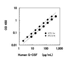
The typical standard curve is shown above. This curve can not be used to derive test results. Please run a standard curve for each assay.
